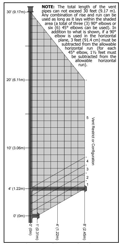
Figure 25. Possible Vent Configurations
